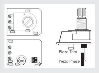
The Fishman Powerchip can be found by opening the round control cover on the lower back of the Hybrid 55. Adjust the small rotary trim pot on the backside of the Powerchip to match piezo and magnetic pickup levels. Move the Phase jumper on the backside of the Powerchip to eliminate phase cancellation between the piezo and magnetic pickups.
